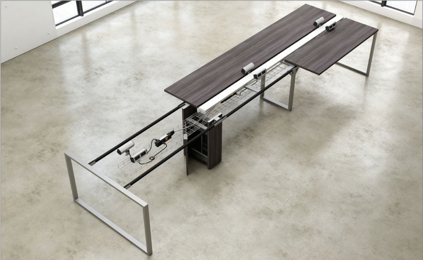
Steel beams running between the support legs give lateral strength to the bench while supporting the worksurfaces. Steel or laminate intermediate legs can be used to provide support for longer runs. The 8-wire, 4-circuit electrical can be placed in the wire basket under the worksurfaces.
