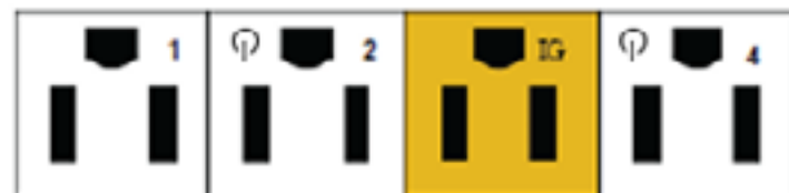
Title-24 Compliant 4-Circuit Block - Circuits 2 & 4 are controlled.
