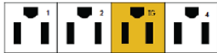
4-Circuit Block - Circuit 3 is an isolated ground
