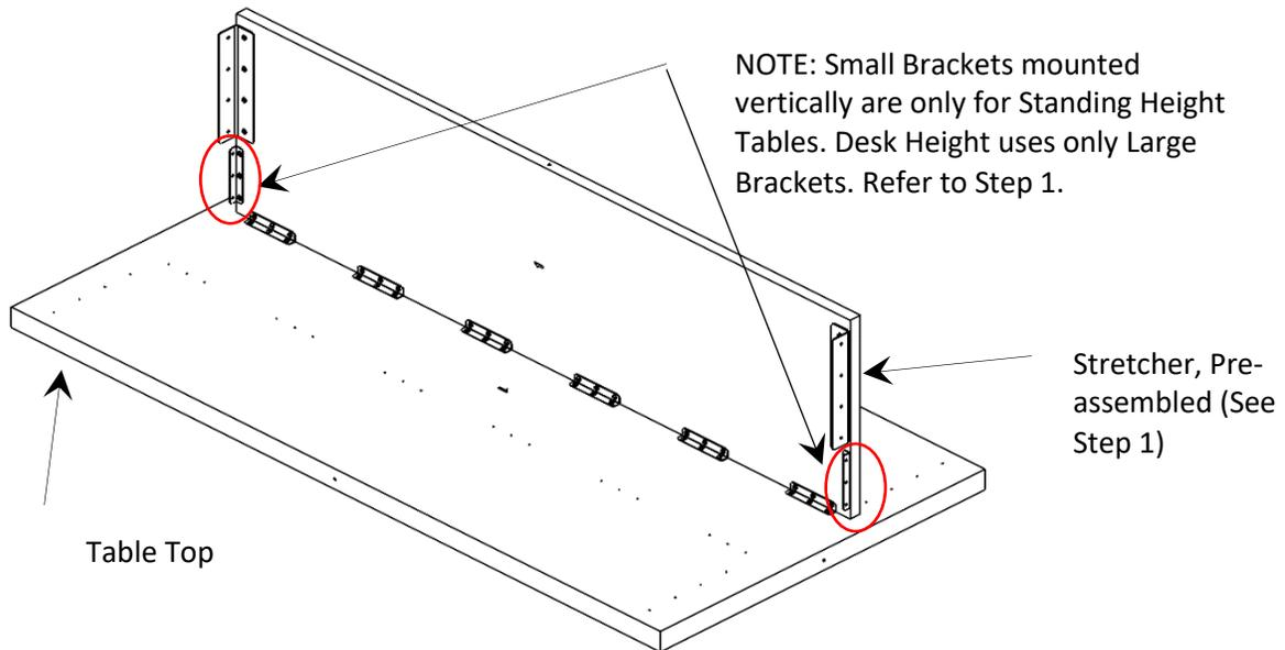
1. Assemble Stretcher as shown using pre-drilled pilot holes on the Table Top. Secure with #8 x 1" L screws. Do not tighten screws at this time to allow movement for final adjustments.
