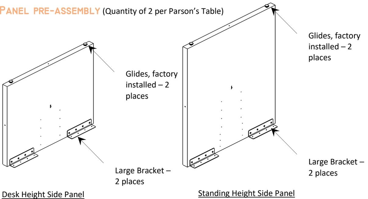
1. Pre-Assemble Large Brackets as shown using pre-drilled pilot holes and secure with #8 x 1" L screws (4 screws per bracket).
