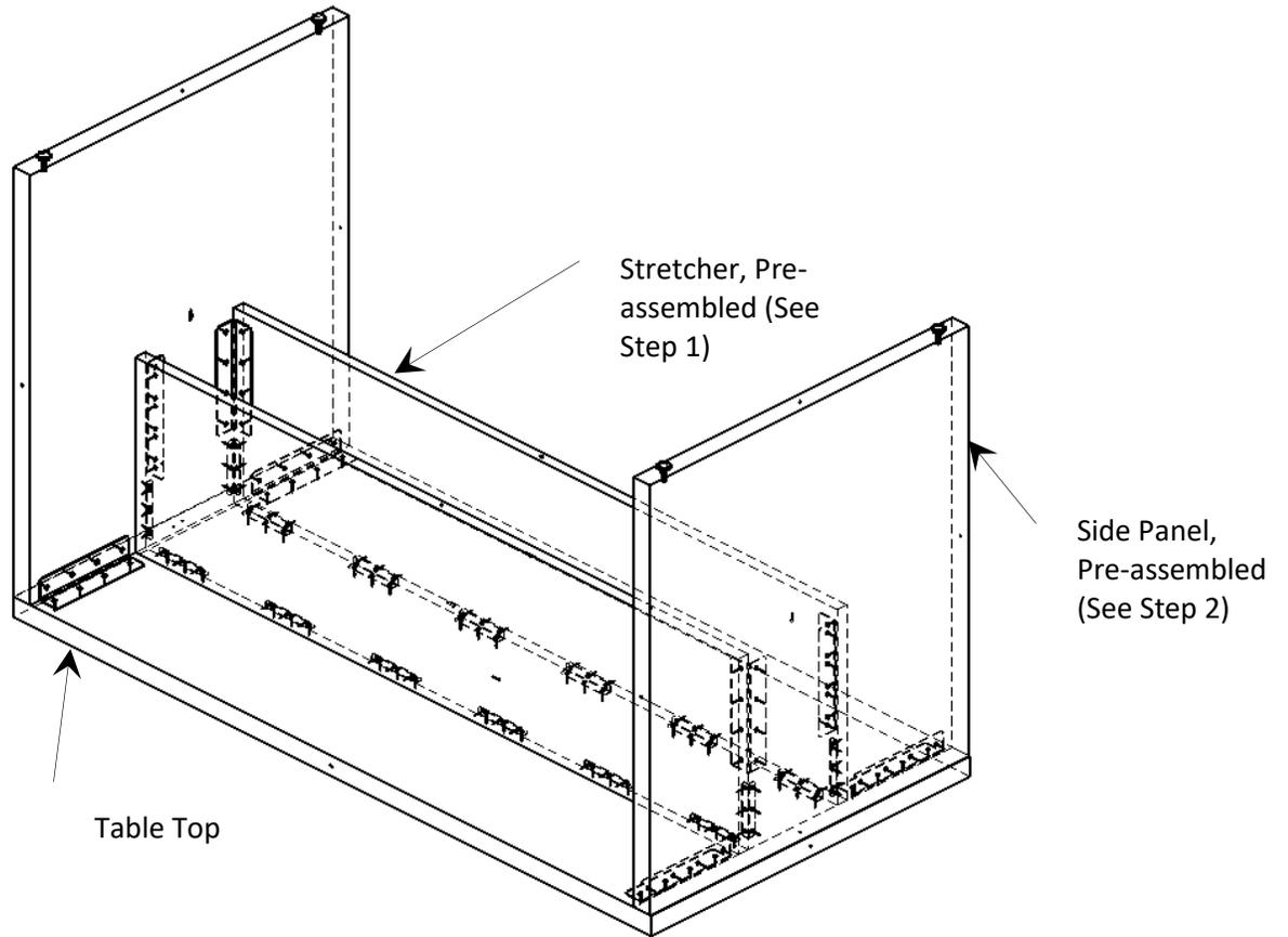
1. Position Stretcher as shown using pre-drilled pilot holes on the Table Top. Secure with #8 x 1" L screws. Align Panels and tighten all screws at this time.
