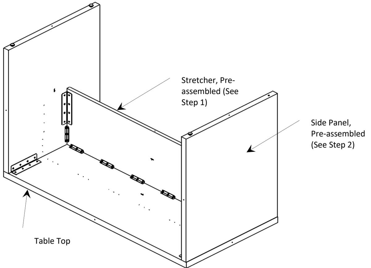
1. Position Side Panel as shown using pre-drilled pilot holes on the Table Top. Secure with #8 x 1" L screws. Do not tighten screws at this time to allow movement for final adjustments.
