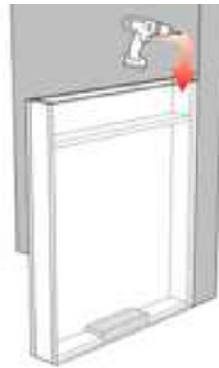
A 2x4 secured to the floor and fitted into the open bottom of the planter wall will steady it, but it still must be attached to a site wall.
